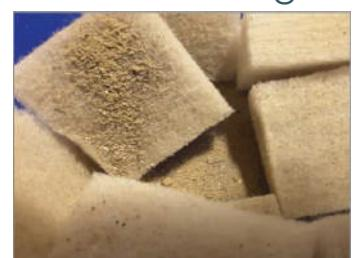
Filtering result after one-time filtration with different flow rates at 1,000 l. extremely contaminated water (100 mg / l) and a particle size of 1-30 microns
